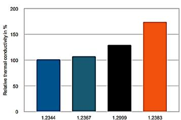
Relative thermal conductivity (Thermodur® 2344 / H13 as a reference) in quenched and tempered condition (45±1 HRc), measured at 100°C.
